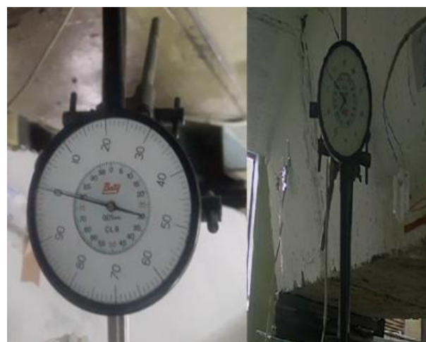
Fig. 7 Dial gauge located at mid-span
