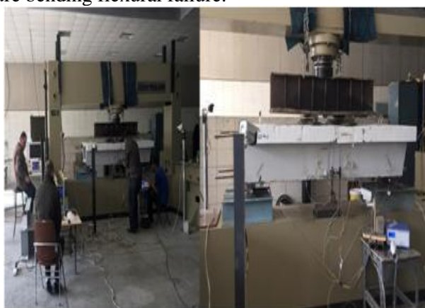
Fig. 6 Testing machine with the capacity of 2500 kN
