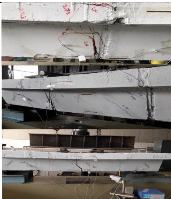
Fig. 11 Failure crack patterns of specimens 1, 2, and 3 for group 1 (Bending failure)
