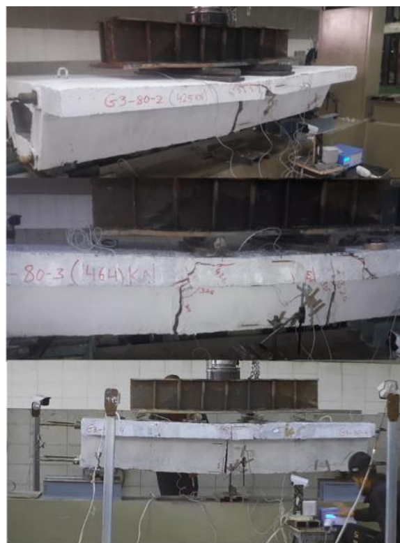
Fig. 12 Failure crack patterns of specimens 4, 5, and 6 for group 2 (Bending failure)
