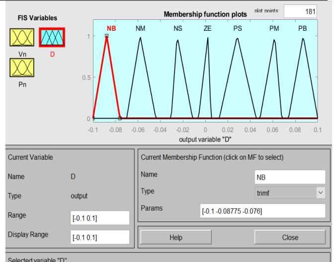
Fig. 15 MFs of the input and output variables for fuzzy logic MPPT
