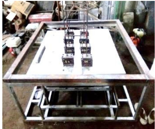
Fig. 14 The shaking table was attached to the base isolator supports through bolted connection
