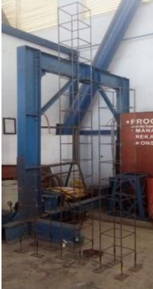
Fig. 11 Three steel frame model prototype specimens for (a) 5 storeys; (b) 10 storeys; (c) 15 storeys
