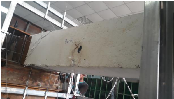
Fig. 9 Failure zones in B-24 (left) and B-25 (right)
