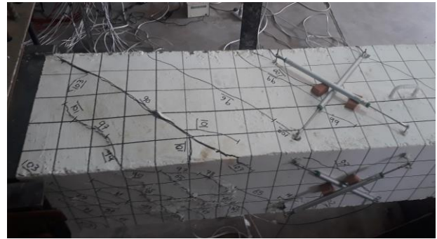
Fig. 9 Failure zones in B-24 (left) and B-25 (right)
