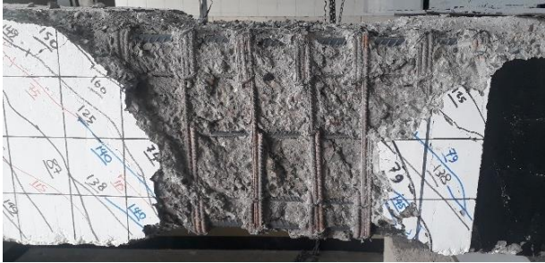
Fig. 8 Failure zones in B-20 (left) and B-23 (right)
