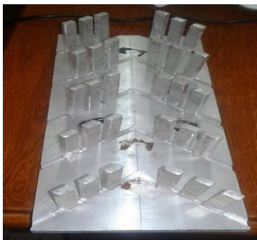
Fig. 1 Interrupted V-type fins
