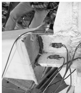
图 10 支撑端部明显滑动(±10 mm) Fig.10 Obvious slippage of the BRB
