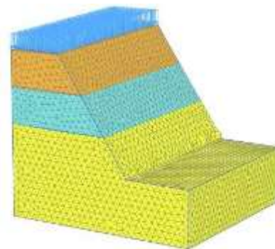
Figure 11. Deformed mesh at optimum moisture content of 19.25%
