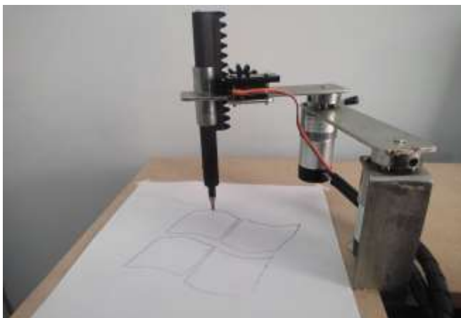
Figure 21. Result of the Windows logo tracing with the physical 2R robot (Authors)
