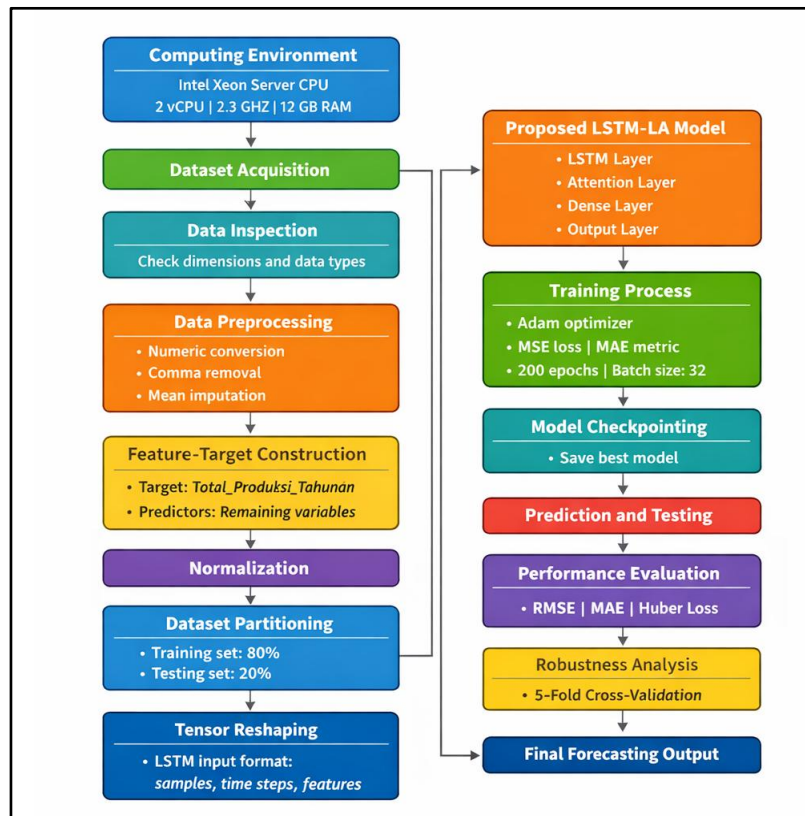
Figure 4. Technical setup for proposed LSTM-LA
