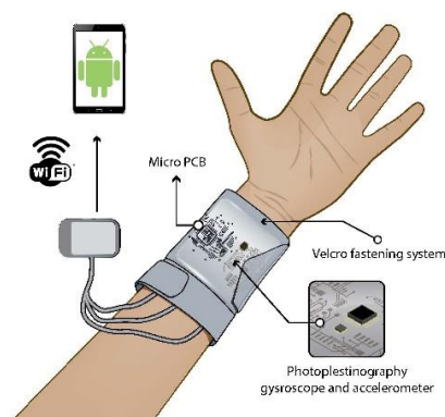
Figure 3. Wearable device overview. Image of the forearm-worn wearable device prototype used for capturing physiological data, including heart rate, SpO 2 , temperature, and motion. It shows sensor placement and communication modules embedded in the device.
