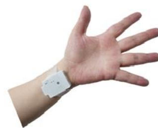
Figure 5. The image depicts a practical implementation of the device on a user's arm. The bracelet-like enclosure securely houses the electronic components and sensors, facilitating comfortable and continuous biometric data acquisition.
