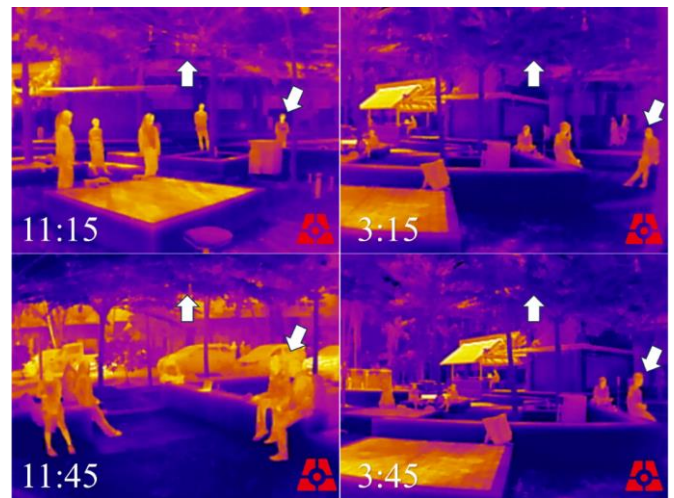
Figure 2. Diurnal thermal distribution of outdoor campus spaces based on infrared imaging (Source: Field measurements)
