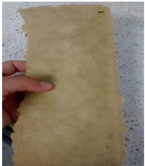
Figure 8. Paper sample with Flecha Caña leaves in 15% sodium hydroxide. Source: Research team
