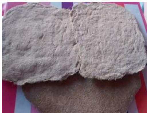
Figure 9. Paper samples of Flecha Caña waste with 5% NaOH, 15% CaO, and 20% CaO solutions.
