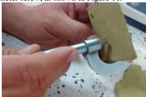
Figure 10. Measuring the thickness of the samples (Source: Research team)
