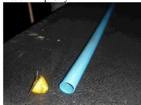
Figure 5. Sampling tube (The authors’ elaboration)
