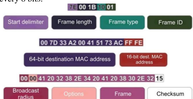
Fig. 18 Data transmission frame between Sensor Node A and the motor node (The authors)
