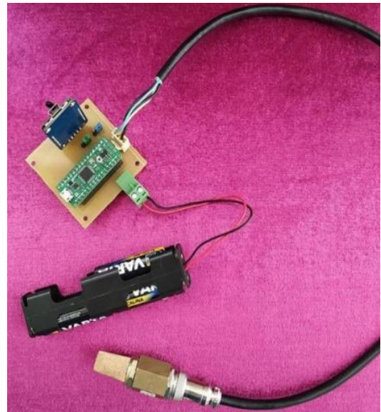
Fig. 17 Implementation of one of the nodes, Arduino Nano and XBee S2C (The authors)
