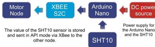
Fig. 5 Block diagram of the sensor node (The authors)
