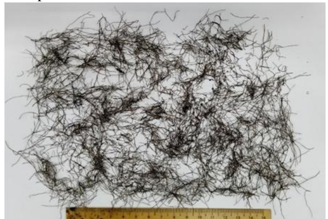
Fig. 2 Waste tire metal fiber used in this study (Developed by the authors)
