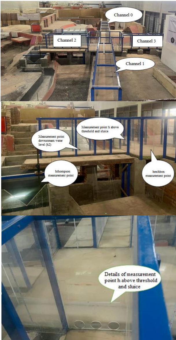
Fig. 7 Details of observation points in the development of model tests (The authors' observation results, 2024)
