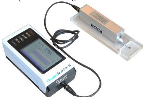
Fig. 2 Equipment used to perform surface roughness measurements
