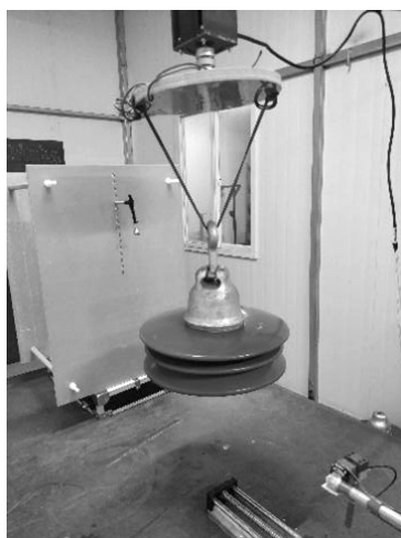
图 8 绝缘子表面电位测量平台 Fig.8 Insulator surface potential measurement platform
