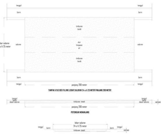
Fig. 5 Canal-blocking design of back filling
