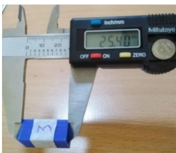
Fig. 8 Measuring the external dimensions of a compression specimen using a digital caliper (Developed by the authors)
