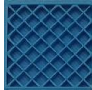
Fig. 5 A slice of a specimen with a rectangular infill (Developed by the authors)
