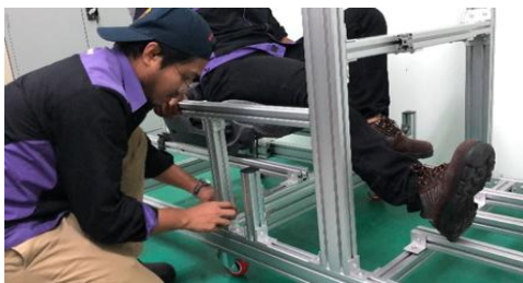
Fig. 13 Assembly procedure for gear lever frame installation
