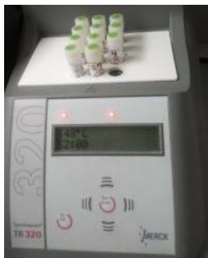
Fig. 3 Spectroquant® TR series thermoreactor, MERCK. TR320 model.
