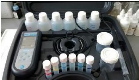
Fig. 2 HACH sensION + 5059 portable potentiometer, multi-parameter electrode: pH, conductivity and temperature
