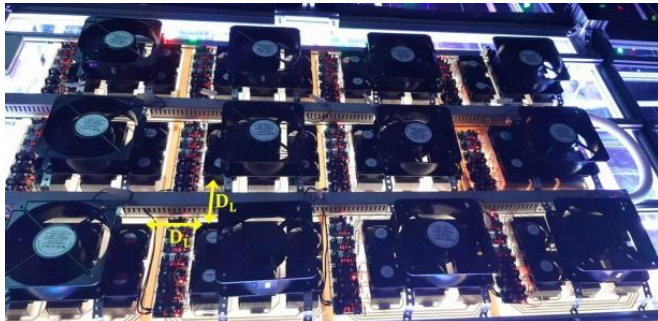
Fig. 4 Top view of the LED array under operation. DL is the distance between the lighting areas of the LED module
