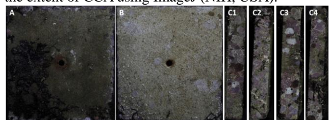
Fig. 3 Settlement plate size 10 x 10 cm has been used for research. A is the upward area, B is the downward area, and C (1-4) is the side area
