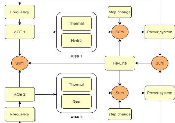
Fig. 1 Schematic diagram of (two-area four-units power system)
