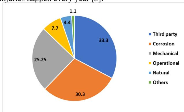
Fig. 1 Percentage of causes of damage in oil and gas pipeline [4]
