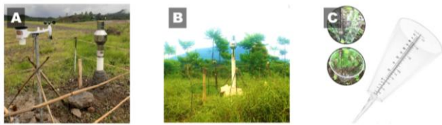
Fig. 3 (a) Manual rain gage and automatic mini-weather stations; (b) manual rain gages in forest plantations; (c) conical funnel instruments (Developed by the authors)
