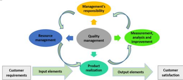
Fig. 6 Model of a process-based quality management system
