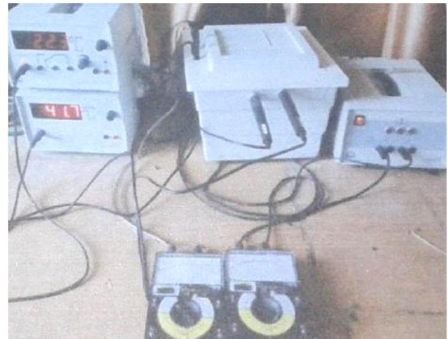
Fig. 1 Thermal conductivity meter with hot square technology ASTM C177
